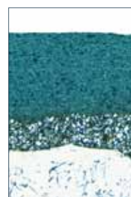
Cross section of Flygt epoxy coating
